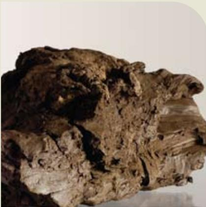
All our raw clay is carefully prepared, milled and left to sour to ensure complete consistency. Once pressed, tiles are dried using the recycled heat from our kilns, before entering our energy-efficient, continuous tunnel kiln to be fired at a consistent and precise temperature.
